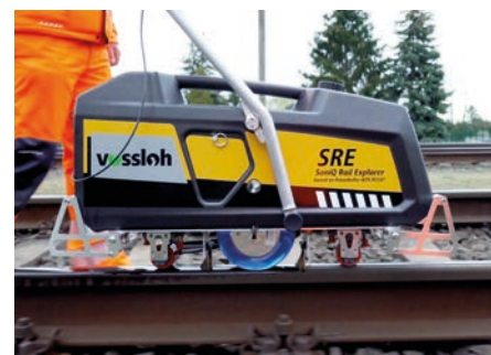
The SRE is ready for use on the track and offers a high test comfort due to its ergonomic design (Source: Vossloh Rail Services).
